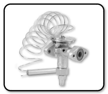
Cold storage plants often have large centralized ammonia systems consisting of many evaporators connected to one or more large compressors. This makes for fairly stable suction pressures. The R/S type L charge responds more quickly to changes in bulb temperature, allowing for a quicker pull-down of the conditioned space temperature. Therefore, for large ammonia systems consisting of multiple evaporators, the Type L charge is recommended.
